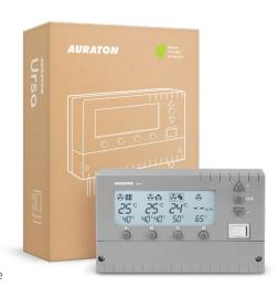
the support of a central heating pump will be used as a heat buffer. AURATON Ursa is equipped with an LCD display with current work readings. Also, the screen is divided into 4 parts, each of which handles a separate device. The controller has an AntiStop function, which prevents the impeller of an unused pump from seizing up.
